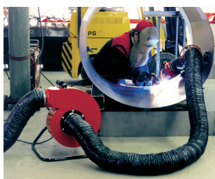
Portable fan working with a magnetic hood during the welding process.
