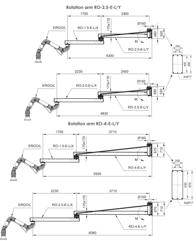
The WB-RO/L bracket serves to install the extension arms – RO-1,5-E-L/X; RO-2,5-E-L/X. Wall bracket does not constitute standard equipment of the extension arm – it has to be ordered separately.
